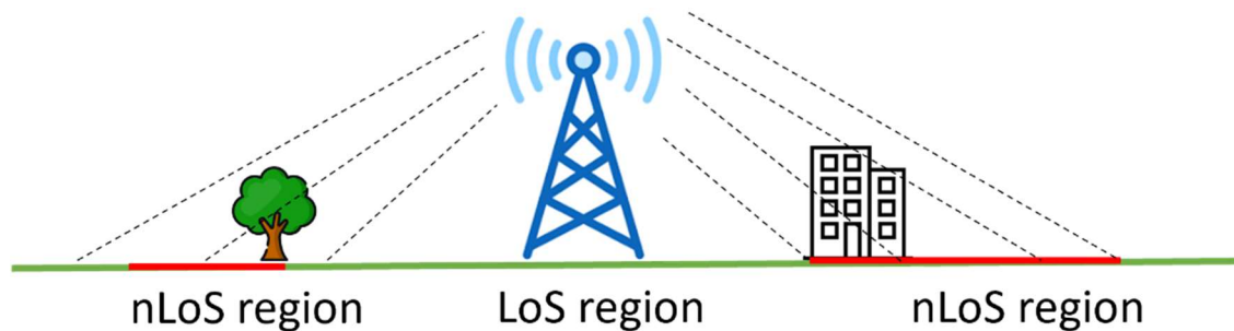
Figure 3: Schematic of LoS and NLoS configurations
